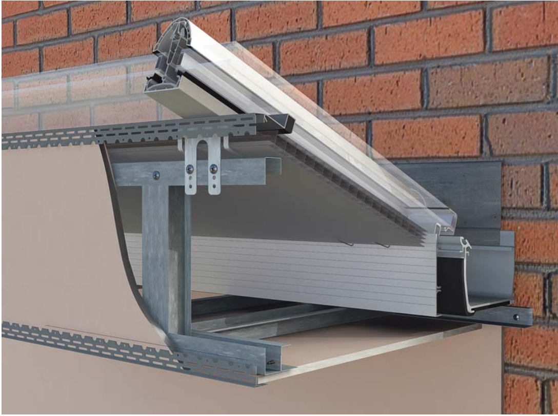
Framework terminates on host wall.
